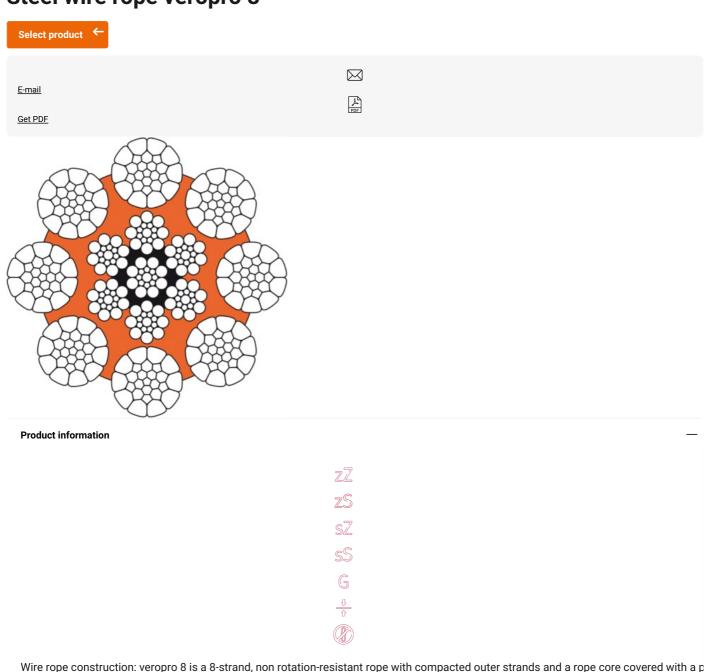
Wire rope construction: veropro 8 is a 8-strand, non rotation-resistant rope with compacted outer strands and a rope core covered with a p
