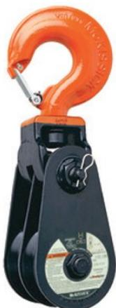
The McKissick snatch block 408 Light Champion from Crosby is a double sheave snatch block fitted with a hook. Available from WLL 4 up to 12 T. Delivered with bronze bushing (BB) and from WLL 12 T also available with roller bearing (RB).
