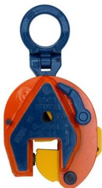
The IPU10A vertical lifting clamp is used for lifting, moving or vertical transfer of sheet, plates, or fabrications. The IPU10A **automatically clicks on to the material** as soon as the clamp is placed on the plate. The fact that the safety lock remains in position as the clamp closes precludes hazardous situations. Fastening the clamp in places that are difficult to reach is no problem.
