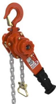
The Hackett L5 QP lever hoist incorporates the four pawl mechanical engagement functionality. The unique and patented pawl design enhances the capabilities of the hoist allowing all four pawls to engage with the ratchet gear in an offset configuration allowing finer adjustment and tensioning capability while maintaining pawl/ratchet engagement. This improves the hoists:
