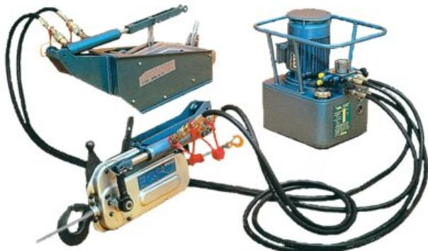
Hydraulic Tirfor machines are portable motorised hoists used with maxiflex wire rope. They can be used to lift, pull and position loads over great distances depending on the wire rope length. They are suitable for use in numerous configurations and are the ideal solution for use in professional applications; they are operated by an hydraulic cylinder powered by either an electrical power pack or a petrol motor power pack
