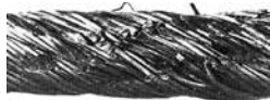
Mechanical damage caused by contact of the running rope with a sharp edge
