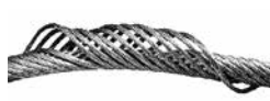
Bird caging after shock load or twisting of multi-layer round strand ropes
