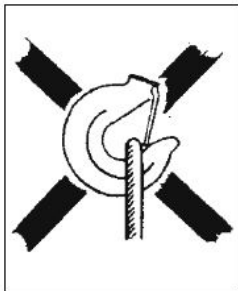
Fig 4 a The sling is applying load to the hook tip!
