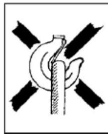
Fig 2 c Hook latch obstructed
