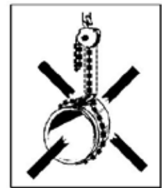
Fig 2 e Load chain must not be used as a sling
